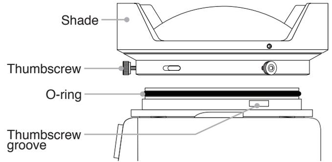
7. Press the port firmly towards the housing until the base of the port is almost flush with the housing front. If there is resistance, remove the port and re-check that the thumbscrews are loosened and that the o-ring is properly lubricated.
