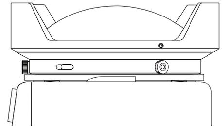
8. Tighten all three thumbscrews while holding the port firmly towards the housing. The thumbscrews should thread in completely until the head touches the port. If the screws are difficult to turn and/or they bottom out before their heads are flush, it is an indication that the port is not pushed far enough down on the housing.
