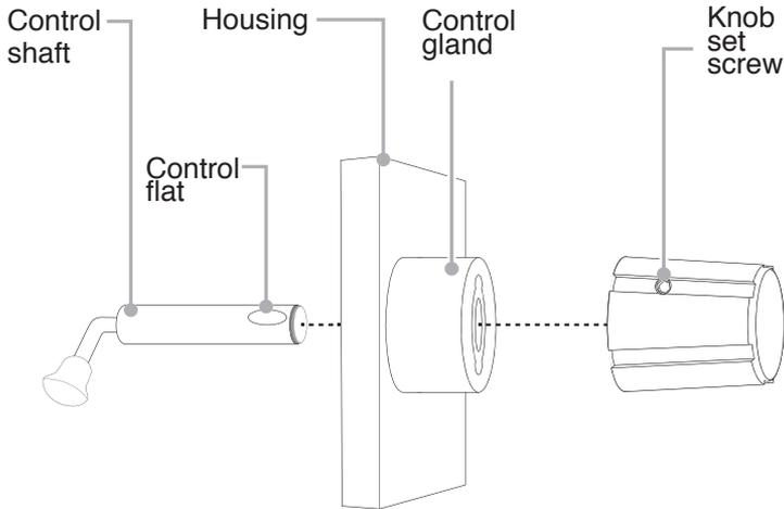
5. Re-install the shaft from the inside of the housing. Rotate the shaft gently for smooth installation into the gland. Push the control shaft all of the way through until the flat of the shaft is visible on the outside of the housing.
