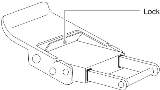
2. Lid snaps are designed to provide enough force to compress the o-ring for a proper seal. Keep firm pressure against the lid snap while lifting it away.
